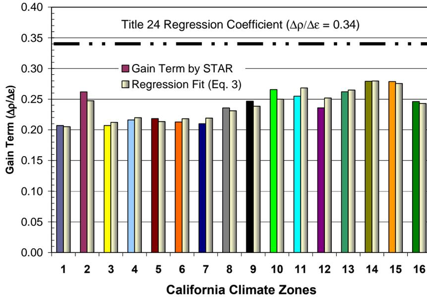
Figure 1. The gain term  $\frac{\Delta\rho}{\Delta\epsilon}$  derived from STAR simulations using the Table 1 pairs of reflectance and emittance for the sixteen climatic zones in California.
