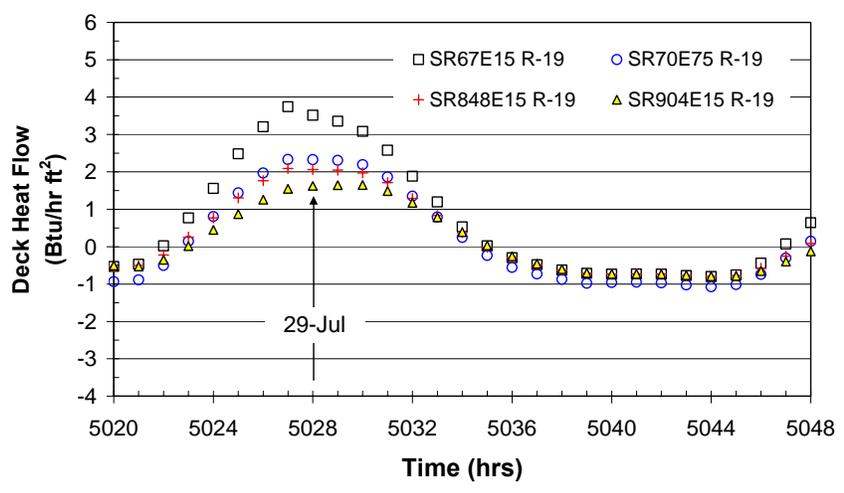
Figure 2. Roof surface temperatures and deck heat flows for Sacramento, CA with acrylic coated Galvalume® having SR67E15 and SR848E15 and the 2005 Title 24 (SR70E75).
