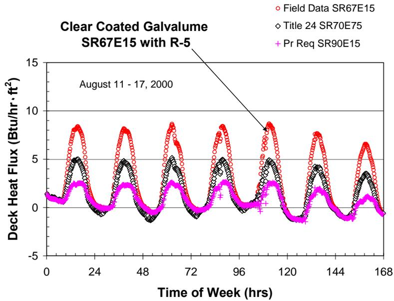
Figure B3. The deck heat flow observed for the acrylic coated Galvalume® roof (SR67E15) as compared to the 2005 Title 24 (SR70E75) roof and the minimal solar reflectance roof (SR90E15).
