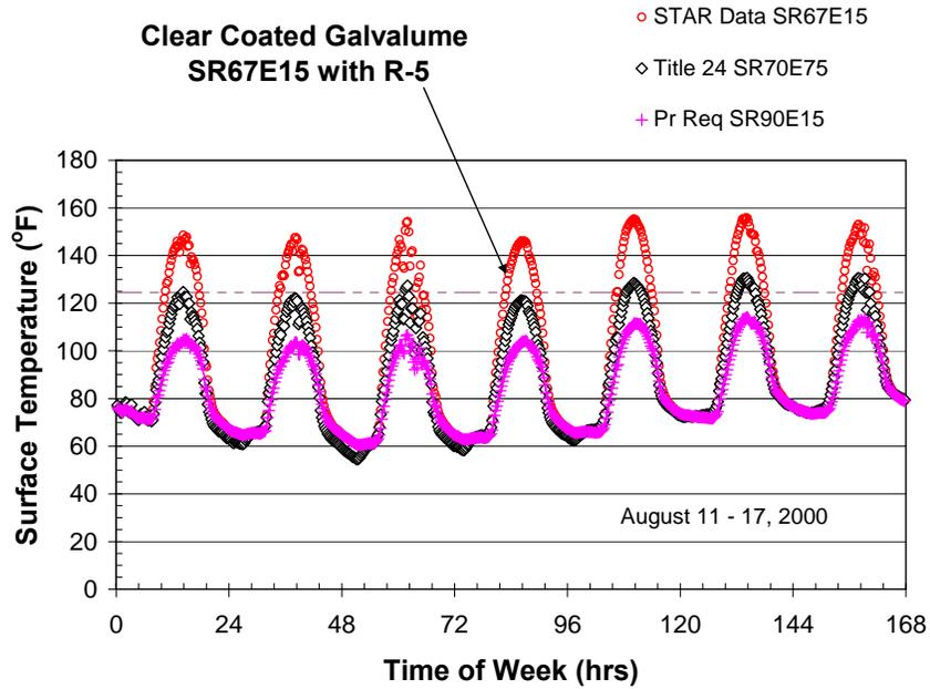
Figure B2. Surface temperature for the acrylic coated Galvalume® roof (SR67E15) as compared to the 2005 Title 24 (SR70E75) roof and the minimal solar reflectance roof (SR90E15).
