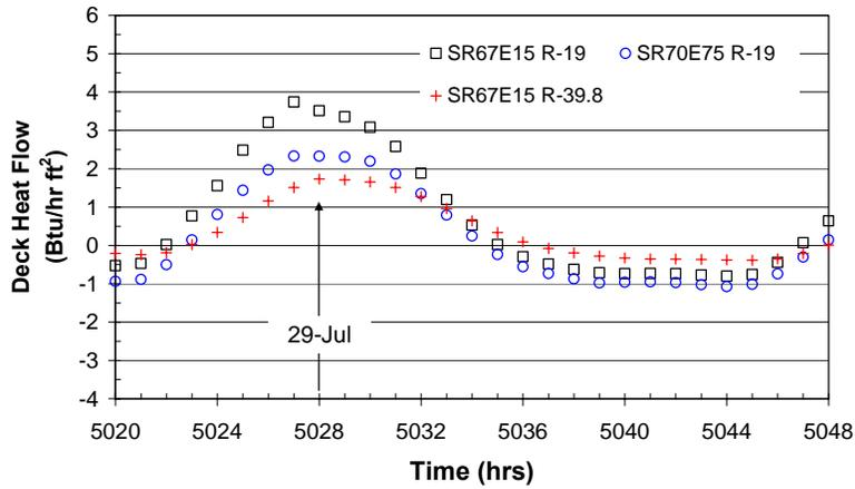
Figure 3. Roof surface temperature and deck heat flows for Sacramento, CA with acrylic coated Galvalume® (SR67E15) having R-19 and R-39.8 levels of roof insulation are compared to the 2005 Title 24 base case (SR70E75).
