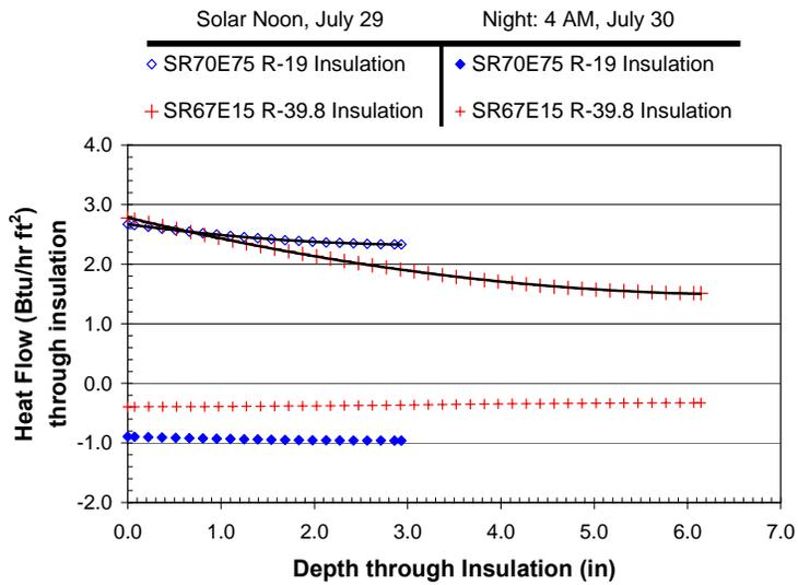
Figure 4. Heat flows at discrete depths into the polyisocyanurate insulation for SR848E15 (R-19) vs the SR70E75 (R-19) and SR67E15 (R-39.8) vs the SR70E75 (R-19).
