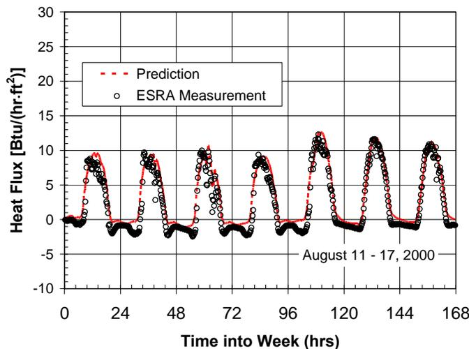
Figure B1. Validation of the STAR code against the measured heat flow penetrating a low-slope roof with acrylic coated Galvalume®.
