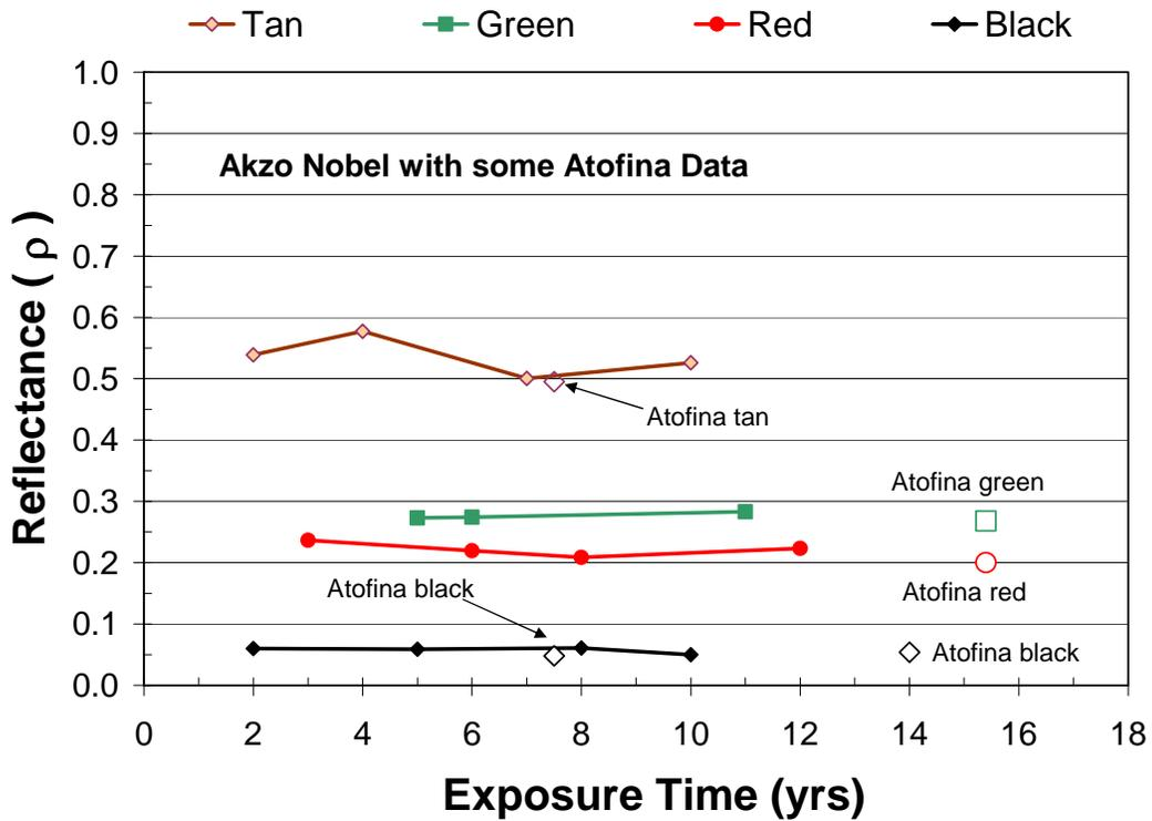
Figure 6. Solar reflectance of Akzo Nobel and Atofina PVDF base paint metal panels over time.
