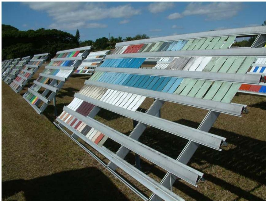
Figure 2. Exposure racks used at Atlas and Q-Lab for exposing PVDF metal roof samples.
