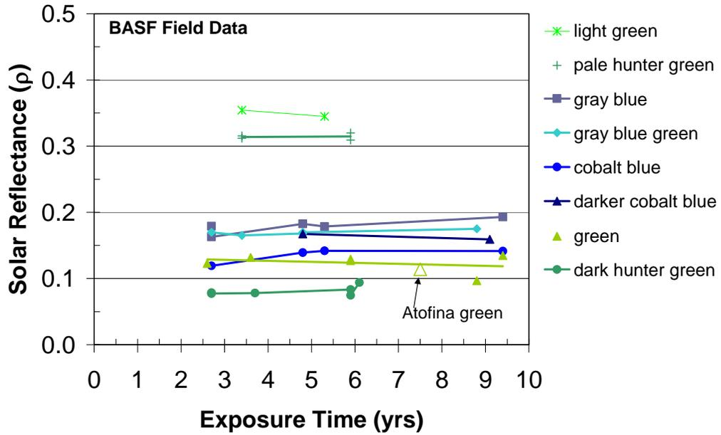
Figure 7. Solar reflectance of BASF PVDF base paint metal over time with Atofina data.
