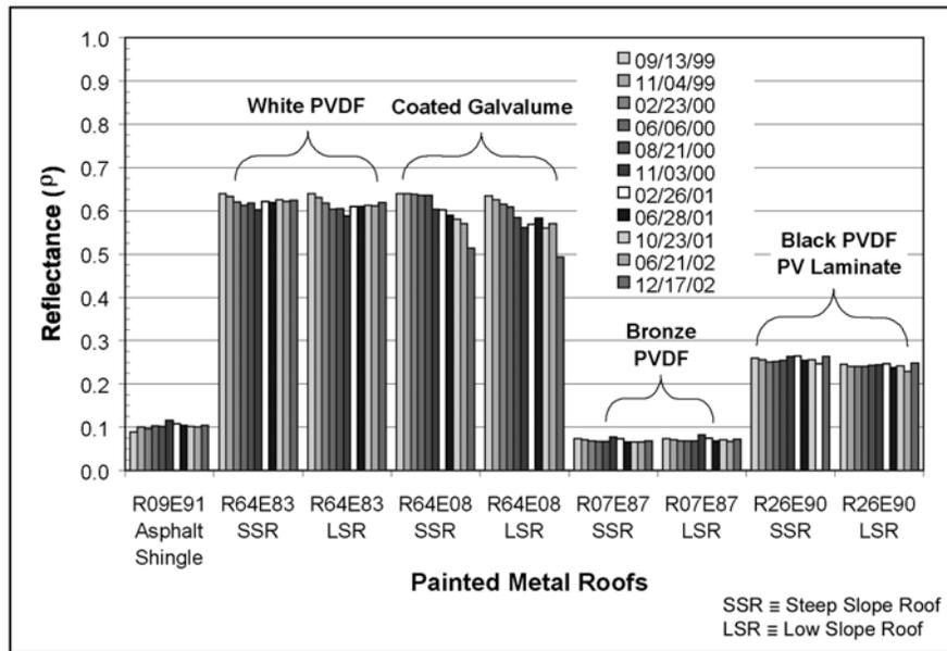
Figure 3. Solar reflectance of the painted metals exposed to east Tennessee's climate on the ESRA.
