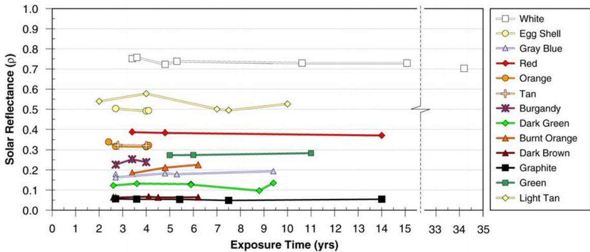
Figure 8. Solar reflectance of PVDF painted metals from BASF, Atofina, Akzo Nobel and Solvay Solexis.
