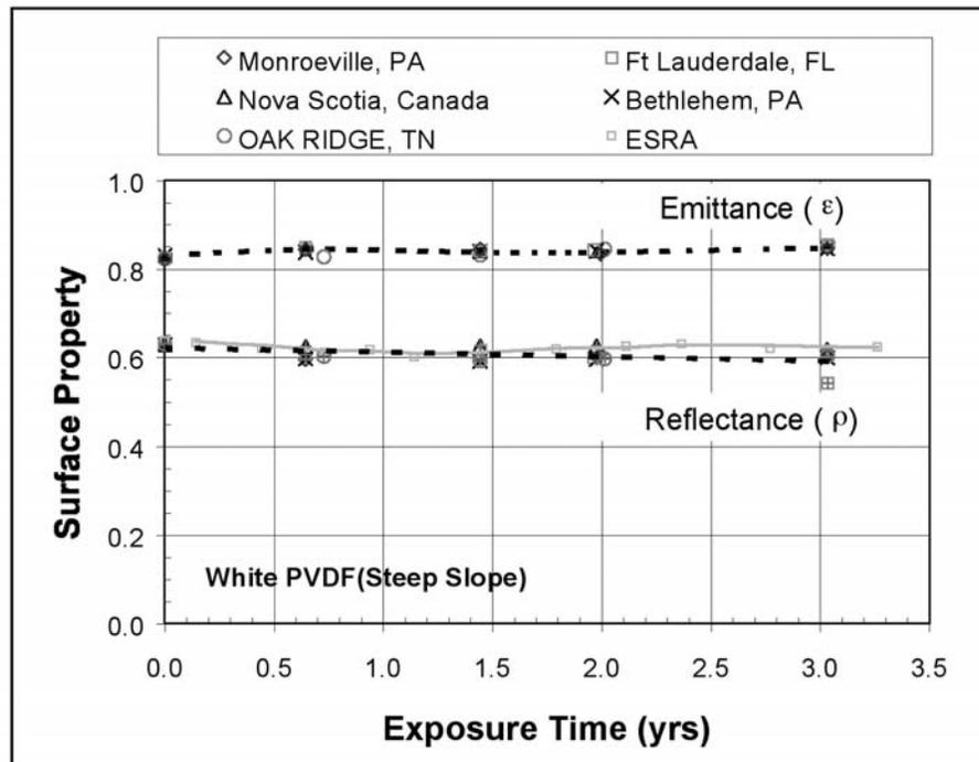
Figure 4. Solar reflectance and infrared emittance of white PVDF painted metal (R64E83) field tested at ORNL.
