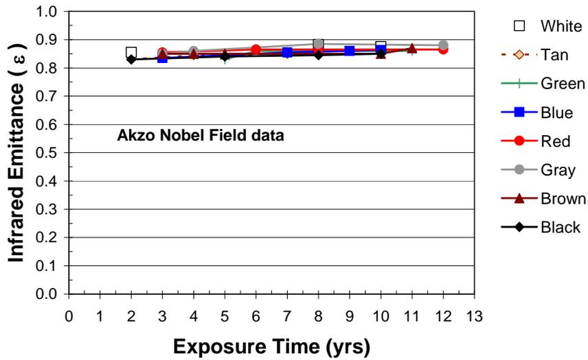
Figure 5. Emittance of Akzo Nobel PVDF base paint metals over time.
